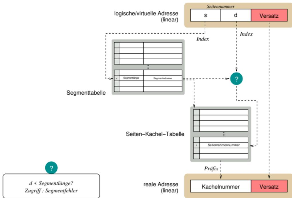
1 SKT =  $la.d < ST[la.s].sd\_limit ? ST[la.s].sd\_base : \text{segmentation violation} \sim trap$
