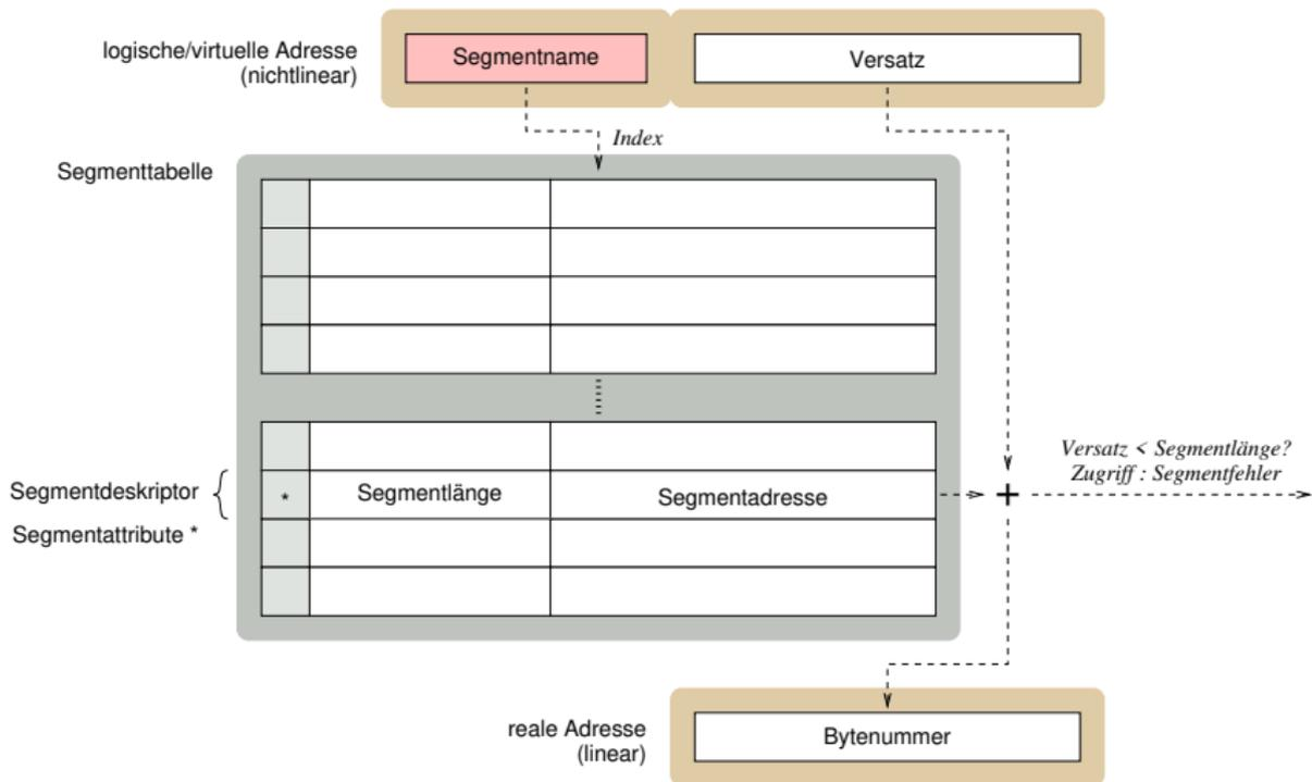
1  $ra = la < ST[sn].sd\_limit ? ST[sn].sd\_base + la : \text{segmentation violation} \sim \text{trap}$
