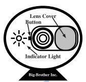
camera controller. When the cover is closed and, thus, the button is pressed, the indicator light should be switched off and the ambient brightness should no longer be queried.
