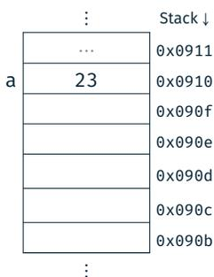
**Caution:** The exact placement of the variable on the stack depends on the compiler and the chosen optimization level!
