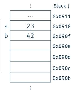
**Caution:** The exact placement of the variable on the stack depends on the compiler and the chosen optimization level!
