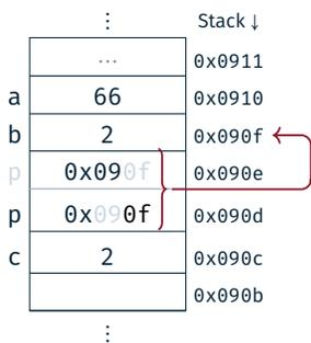
Caution: ATmega328PB has 8-bit registers and 16-bit addresses
